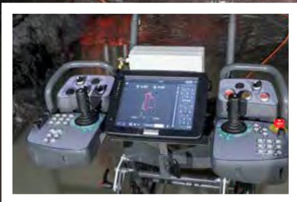
The control system for Sandvik DU412i enables remote operation for tramming, outrigger and levelling operations.
