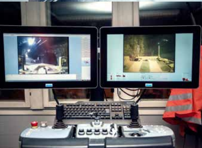
Remotely controlled cameras onboard the equipment enable 360-degree visibility for operators.
