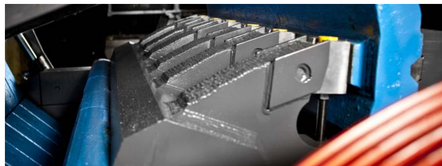
Detail of Prisec™ 3 rotor
