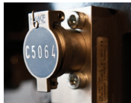
Mechanical safety interlock system
