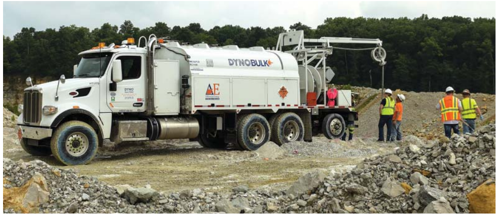
The \Delta E^2 system assimilates data from smart drills and geologic models to optimize blast energy. Users can then custom load each pattern, as well as the individual holes, according to geologic conditions and desired PF. (Photo: Dyno Nobel)
